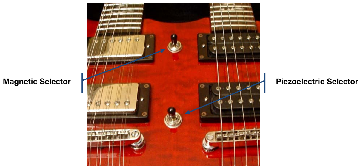
Figure 7 - Selectors for Magnetic and Piezoelectric Outputs
